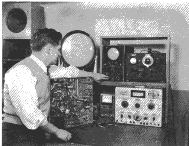
Fig. 98. Alignment using sweep generator with self-contained marker generator.
